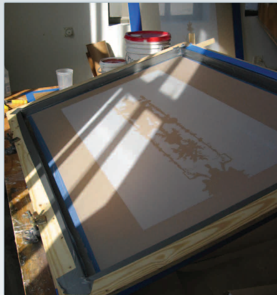
This screen-printed stencil will mask the printed elements of the design while allowing adhesive to be squeegeed onto the background.
