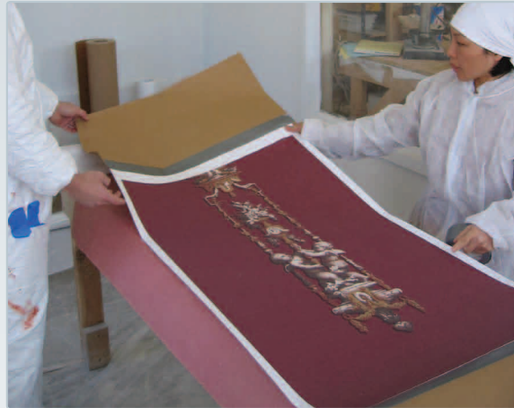
This is the base print from the digital printer for a panel that is to have the background color flocked. Flocking is a technique for attaching finely chopped felt to parts of the paper to create the effect of velvet that was very popular for a time in the nineteenth century.
